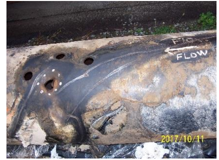
Figure 4: Puncture from Backhoe with Unbarred Teeth
